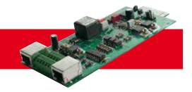
The RS485 card enables the creation of a BUS to connect additional inverters, displaying all parameters via connection to a PC equipped with SunVision software.
